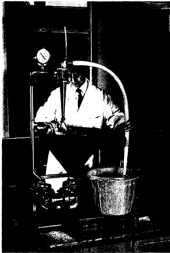
Figure 12. 50 mm hydrocyclone in operation.
